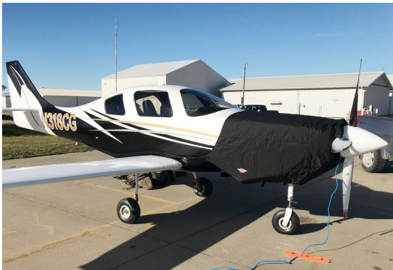
Lancair IV-P Insulated Engine Cover, fully enclosed
