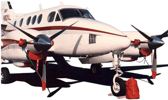
Pitot, Exhaust Covers, Engine Plugs & Prop Ties
