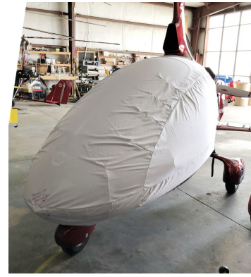
Cavalon Gyrocopter Bubble Cover, test fit cover
