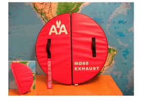
PW JT8D Off-Link Protective Long-term Storage "Rain Cap" Engine Cover
