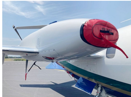
Piaggio P180 Intake Plugs with Fabric Extension
