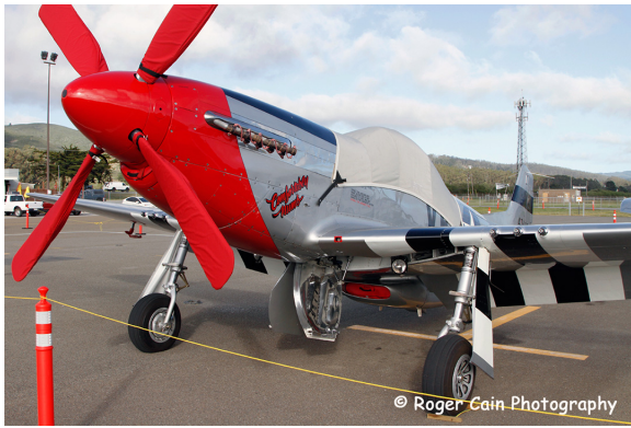
North American P-51 Mustang Canopy Cover, Belly Scoop and Chin Scoop Plugs
