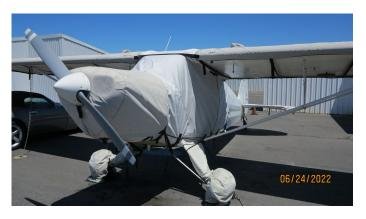
Piper PA-12 Over-Top Canopy Cover, Engine, Wing & Landing Gear Covers
