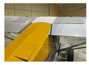
Piper J5A Windshield/Skylight Cover, test fit
