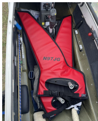
Schempp-Hirth Ventus-2B winglet/wingtip pads
