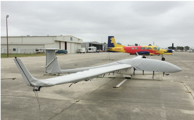
DG-505 Canopy/Nose, Wing, Empennage & Horiz. Stab. Covers
