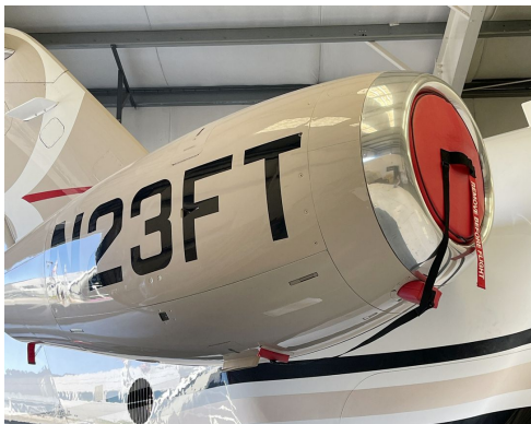
Hawker Beechcraft Premier 390 Intake Plug/Exhaust Plug Set Premier Intake/Exhaust Plug set with Generator Inlet/Exhaust Plugs
