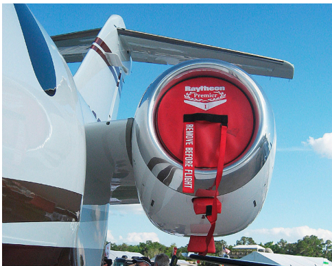
Hawker Beechcraft Premier 390 Intake Plug/Exhaust Plug Set Premier Intake/Exhaust Plug set with Generator Inlet/Exhaust Plugs
