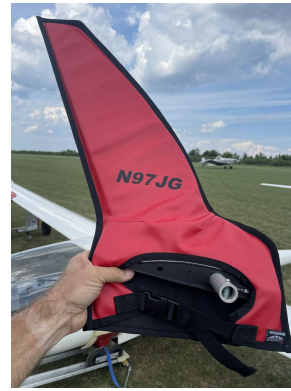
Schempp-Hirth Ventus-2B winglet/wingtip pads
