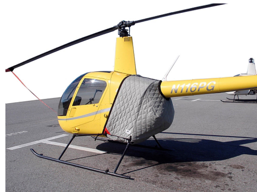
Robinson R-22 Insulated Engine Cover (also covers bottom) & Front Blade Tie-down
