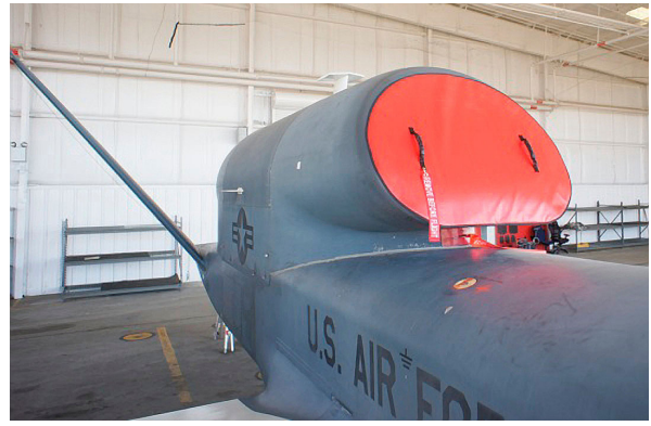
RQ-4/MQ-4 Global Hawk Intake Plug w/ lip (Fits both A & B models & all blocks)
