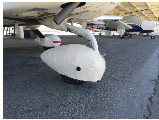
Grumman AA5 Nose Wheelpant Cover, test fit
