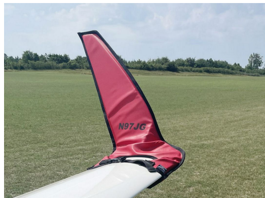
Schempp-Hirth Ventus-2B winglet/wingtip pads
