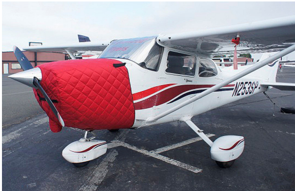
Cessna 172 Insulated Engine Cover, fully enclosed
