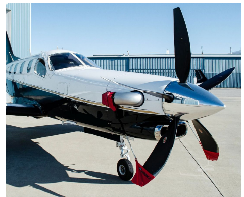
TBM 900 Prop Tie/Exhaust Covers
