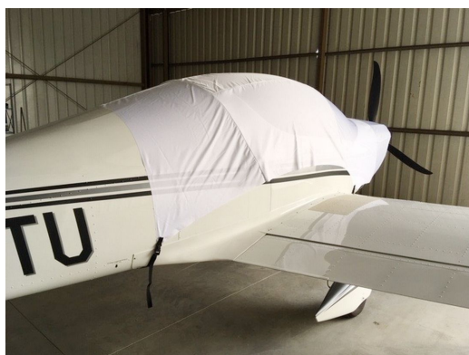
Tecnam Astore Canopy/Engine Cover, test fit cover
