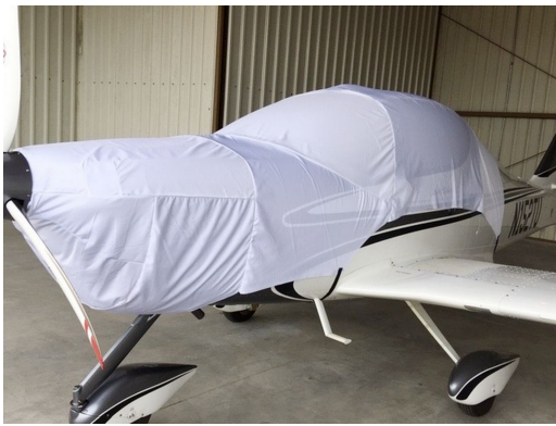
Tecnam Astore Canopy/Engine Cover, test fit cover
