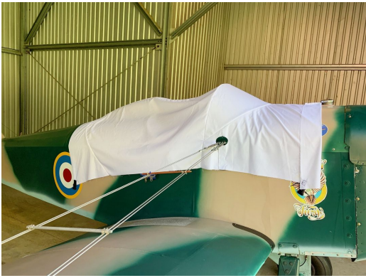
Bowers Flybaby Canopy Cover, test fit design
