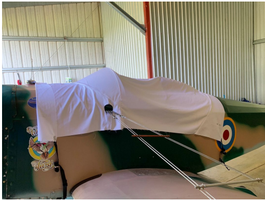
Bowers Flybaby Canopy Cover, test fit design
