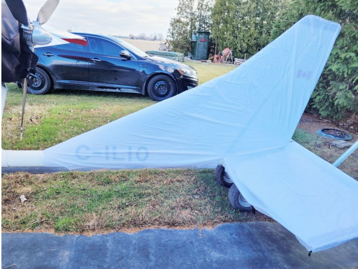
Titan Tornado Empennage Cover, test fit cover
