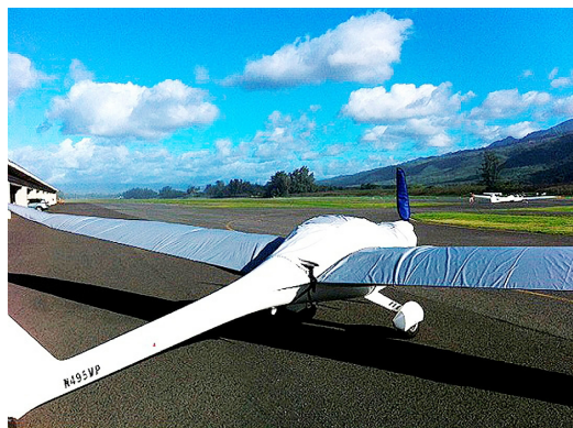
Lambda Canopy/Engine Cover and Wing Covers
