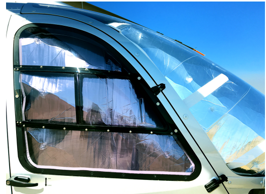
Eurocopter EC-145 Cockpit Heatshields
