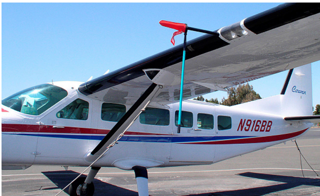
Cessna 208 Caravan Telescoping Pitot (for amphib. models)
