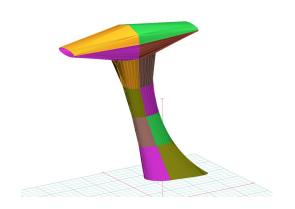
Autogyro Calidus Rotor Mast Cover, 3D model
