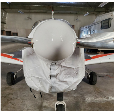
Zlin 142C Engine Cover, test fit cover
