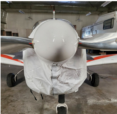
Zlin 142C Engine Cover, test fit cover
